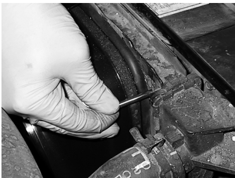
Install temp. probe near inlet hose...
