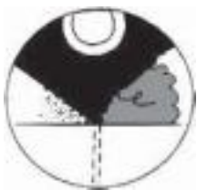
Conventional trimmed lip has sharp edge & rough surface on lube side.
