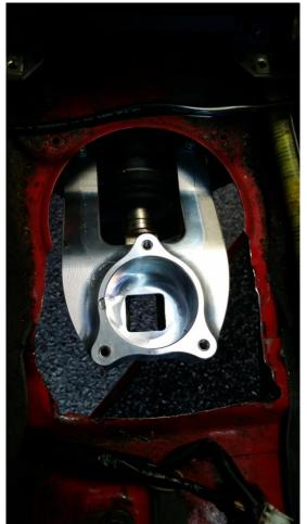
10. Install transmission on engine. Install your old transmission mount on the Z33 transmission and attach to chassis with new crossmember. Install driveshaft and fill trans with oil.
