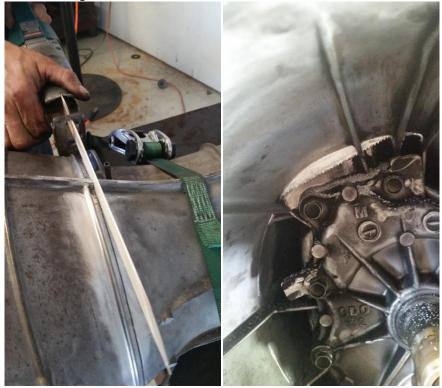
3. Remove bell housing from transmission. Cut off boss according to picture.
