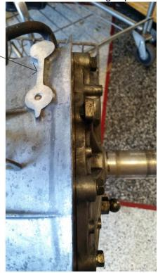
4. Mark and cutoff 3/8" from the input shaft. Chamfer the end of shaft similar to the OEM.
