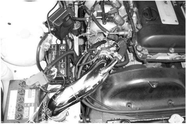
Fit the driver side lower pipe and connect it to the intercooler.
